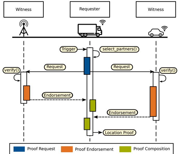
Figure 1: Conceptual overview of the COLAW system. The requester collects location endorsements from witnesses to create a location proof.
