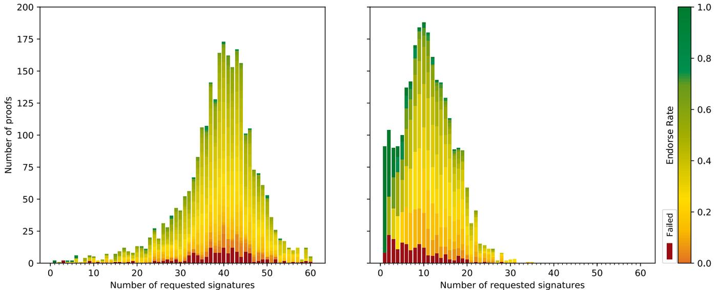
Figure 3: Number of proofs as a function of the number of requested signatures for the reference (left) and the urban scenario (right).
